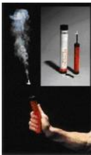
Figure 5: Smoke Pencil Used to Check for Air Leaks
